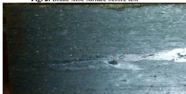
Fig.3: Brake shoe surface after test
